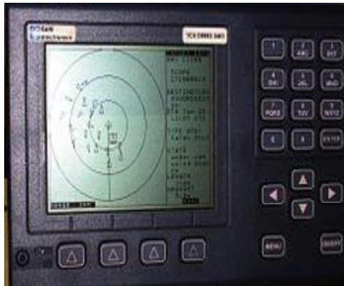
Figure 29: An AIS-equipped system on board a ship, presenting the bearing and distance of nearby vessels in a radar-like display format
