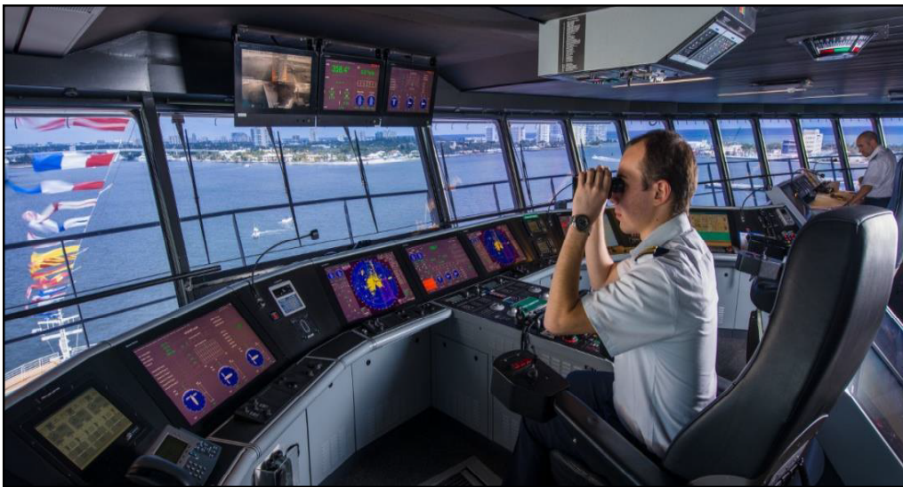
Figure 32: Image of a modern vessel's bridge equipped with IBS
