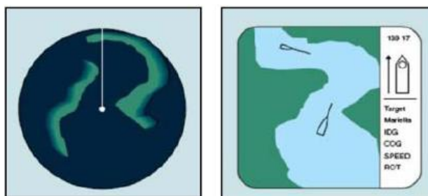
Figure 31: The use of AIS in collision avoidance
