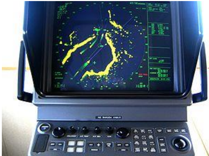
Figure 16: A typical shipboard radar system with ARPA Display of 20 th -21 st century
